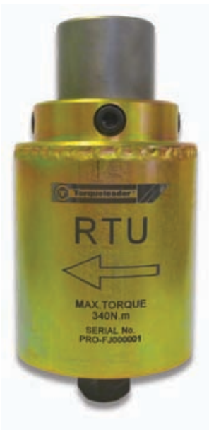
Modification of RTU for Track Bolt Tightening
